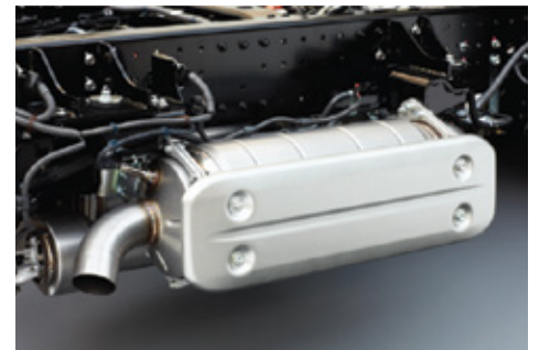
Hino's Selective Catalytic Reduction (SCR) technology substantially lowers harmful NOx and particulate emissions.
