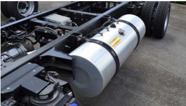
208L (55 Gallon) Aluminum fuel tank, optional component for the Hino model 195.*
